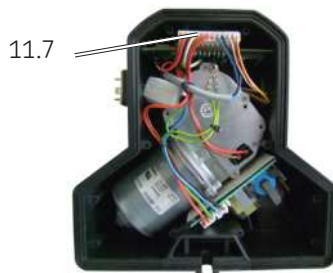
Plug of the control PCB Fig. 25
