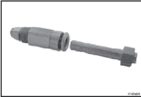
FIG.4 Distributor outlet connector and hose stud with reinforced snap ring
